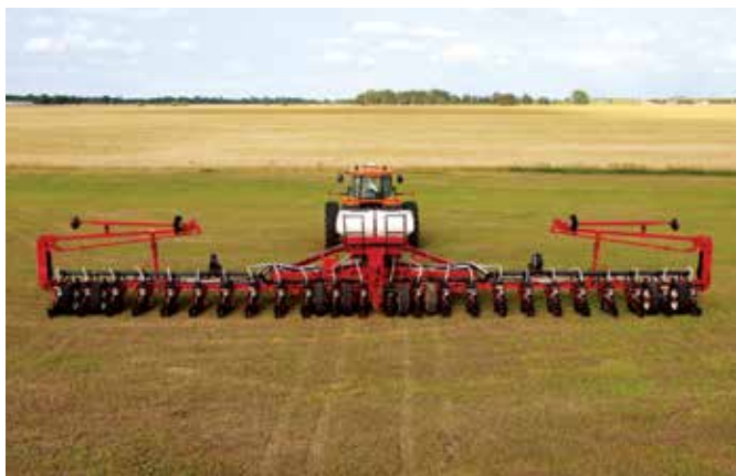
A row-crop planter drops seeds at regular intervals within the row. On newer machinery, electronic monitors count the seeds as they drop and control the seeding rate so that neither too much seed nor too little gets planted.
